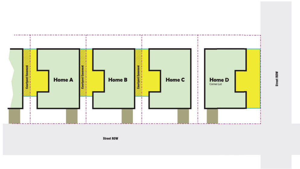
TYPICAL COURTYARD EASEMENT
