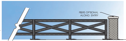
TYPICAL CROSS BUCK HORSE FENCE COLOR TO MATCH YARD ARM AND POST
