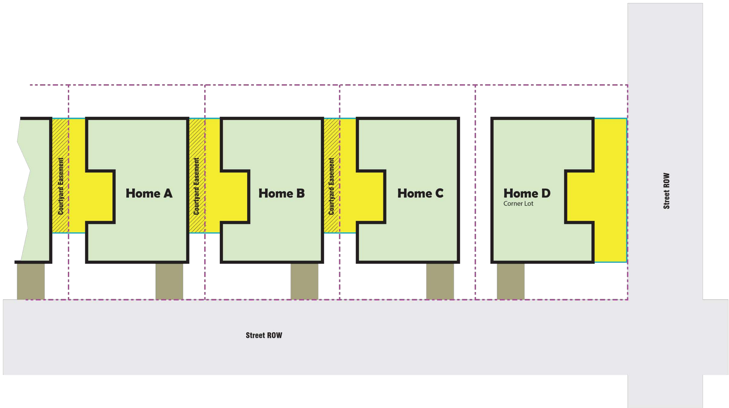
TYPICAL COURTYARD EASEMENT
