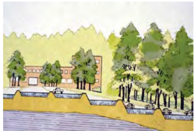
Figure 2: Slope stepping with berms Source: Andronogon
